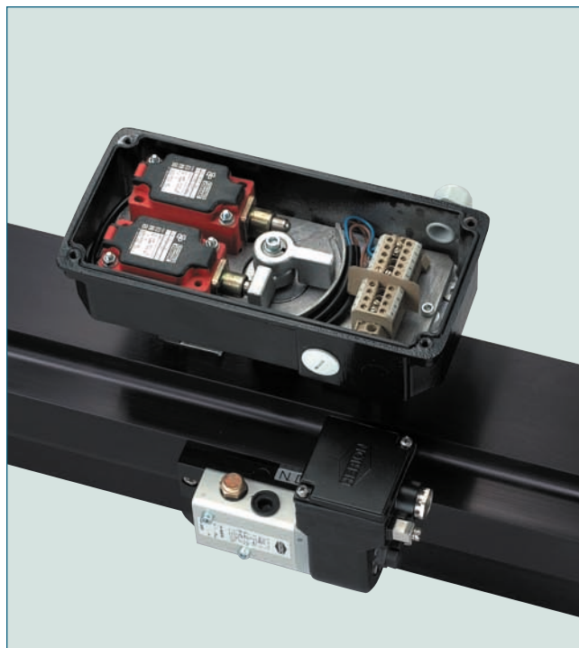
Pneumatic Quarter Turn Actuator (spring returned) with Switchbox MSK (Size II). Integrated mechanical limit switches. Support acc. to VDI/VDE 3845. Pilot solenoid valve for single acting pneumatic actuators.
