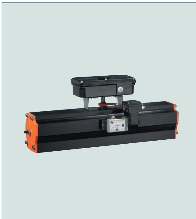
Pneumatic Quarter Turn Actuator (spring returned) with Switchbox MSK (Size II). Integrated mechanical limit switches. Support acc. to VDI/VDE 3845. Pilot solenoid valve for single acting pneumatic actuators.
